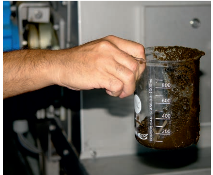
The pump moves 5 to 10 m³/h of abrasive thick sludge with 6% dry substance at a pressure of 8 to 12 bar.
