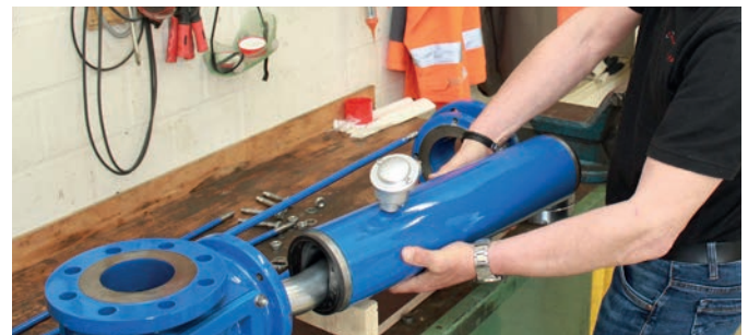
This figure shows how the stator is pulled off.
