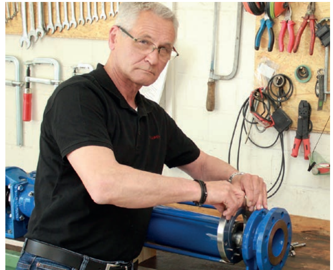
Optifix can be disassembled with just a few motions. Shown here, the screws are already removed so that the removal pieces can be removed in the first step.
