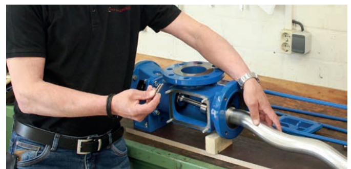
In this image, the inspection cover is removed and how the rotor is then removed.
