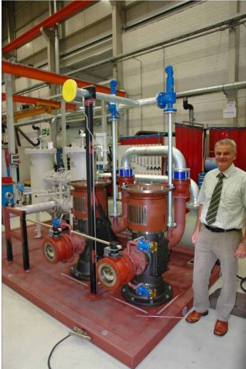
Redundant twin three-screw pumps of the SNS series in an oil-supply system ("OWGX" construction type) for an extruder drive. The pumps move synthetic or mineral oil VG320 at a pressure of 8 bar.
