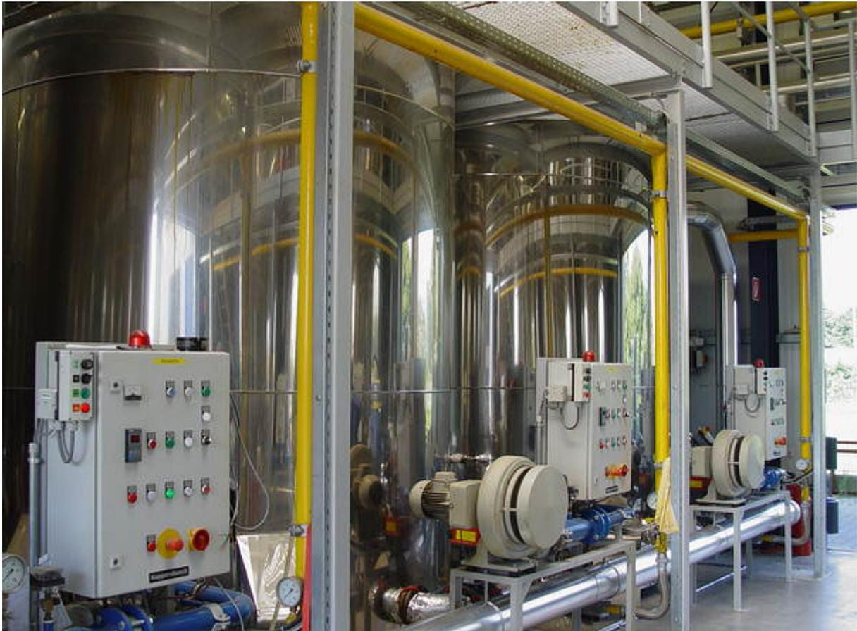
The pumps are mounted on base plates and installed in series. For this reason, they must be capable of precise proportioning and each one must run at the same capacity.
