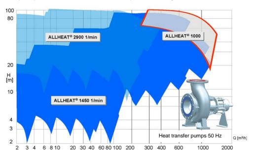
The ALLHEAT family of heat-transfer pumps includes fourteen different centrifugal pump models.
